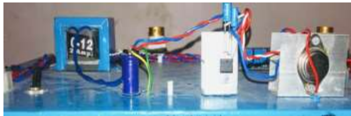
Fig. 5 electrical Power supply
